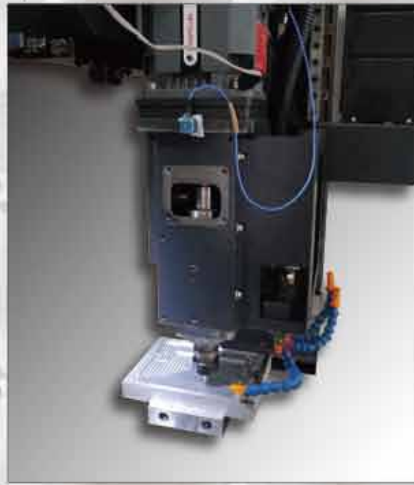
Spindle Vibration Test in Y Direction
